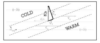
**Figure 1.** Schematic of a region of upper-tropospheric geostrophic cold air advection in cyclonic shear. Thin grey lines are the geopotential height lines, grey vectors are geostrophic winds, and dashed lines are isentropes with cold air on the left. The **Q**-vector is indicated by the open shafted arrow, with its transverse and shearwise components,  $\mathbf{Q}_n$  and  $\mathbf{Q}_s$ , indicated by the bold black arrows. See text for additional explanation.
